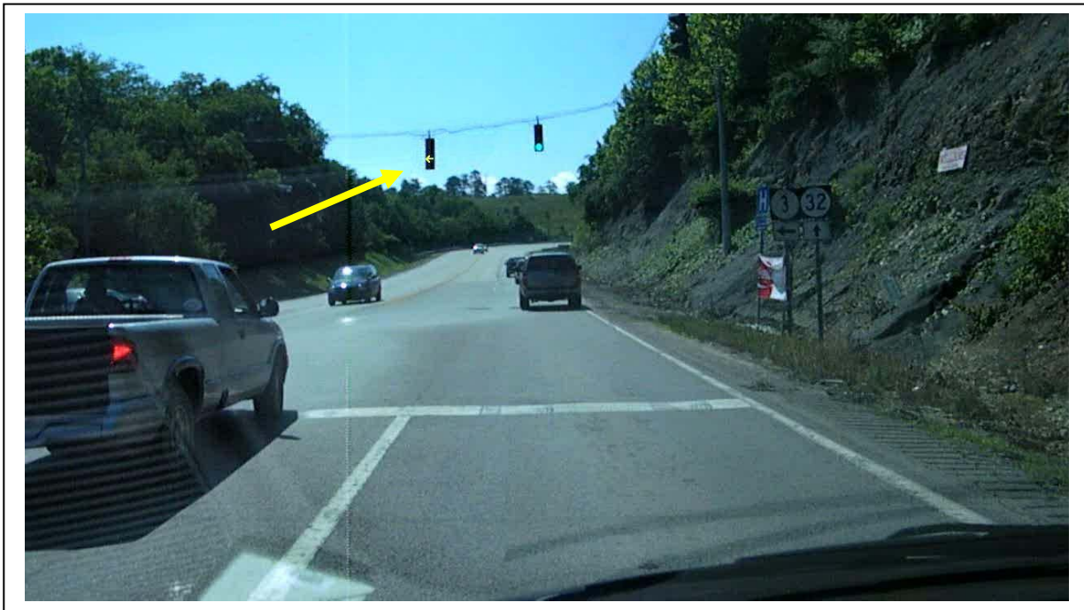
Photo 1: Flashing Yellow (simulation) for Permissive Left Turn
