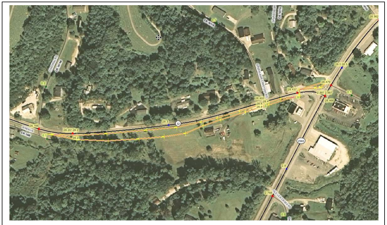
Figure 6: Option 1, Widening existing alignment of KY 32 from MP 28.2 to 28.466
