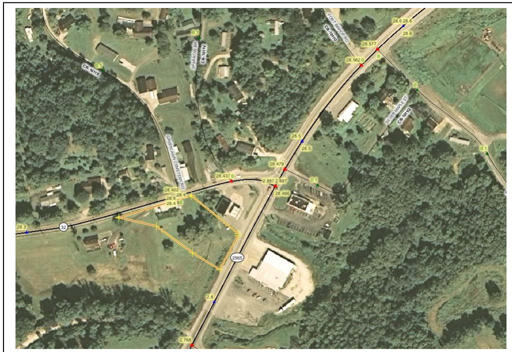
Figure 5: Option 2(Tiii O2), Re-locate intersection
